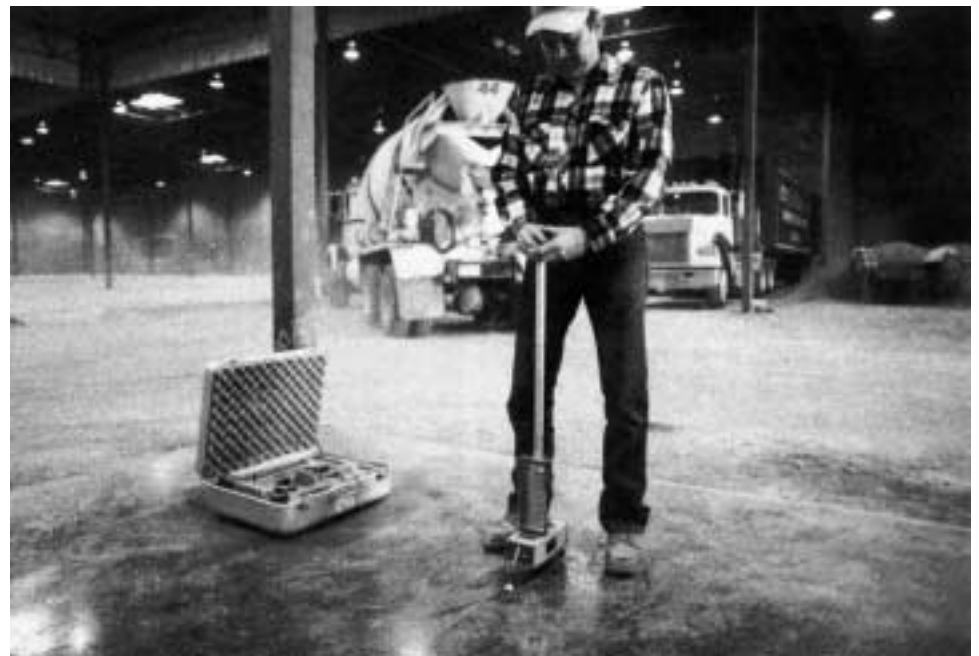
The non-superflat slabs were measured for compliance with the specified F-numbers by taking readings with a Dipstick the morning after placement.
